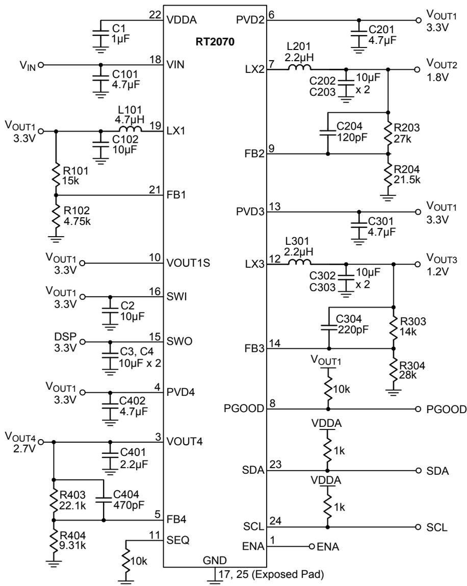
If there is any CHx is not used that external components still must be existed and keep original application circuit.
