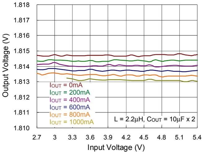
CH3 Buck Output Voltage vs. Input Voltage
