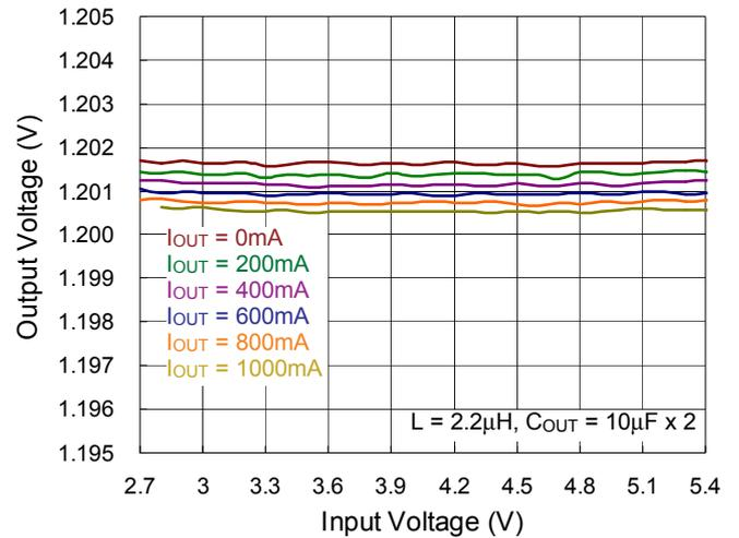
CH4 LDO Output Voltage vs. Input Voltage
