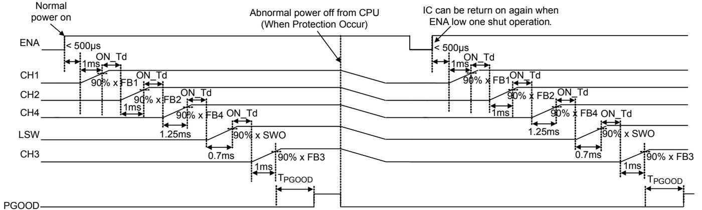
**Note :** ON\_Td and OFF\_Td time control by Register ON\_Td <1:0> and OFF\_Td <1:0> , default setting <00> = 0ms, and T<sub>PGOOD</sub> = 20ms
