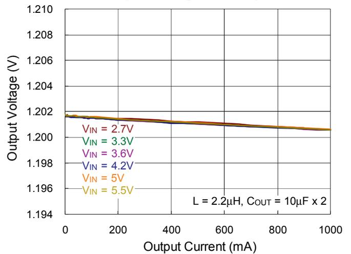
CH4 LDO Output Voltage vs. Output Current
