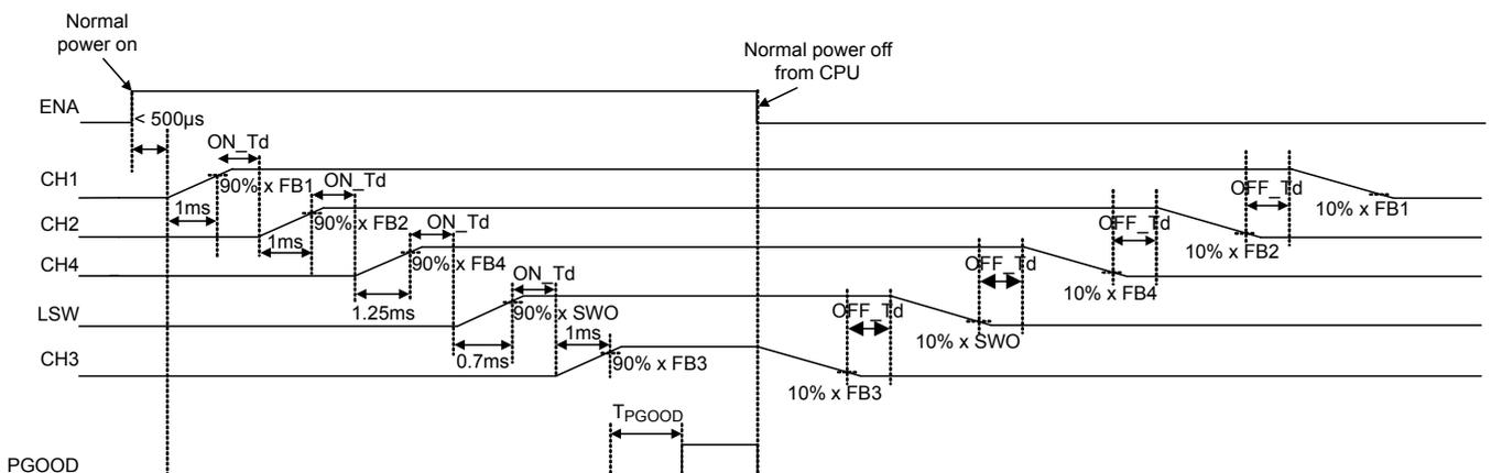
**Note :** ON\_Td and OFF\_Td time control by Register ON\_Td <1:0> and OFF\_Td <1:0>, default setting <00> = 0ms, and T\_PG00D = 20ms
