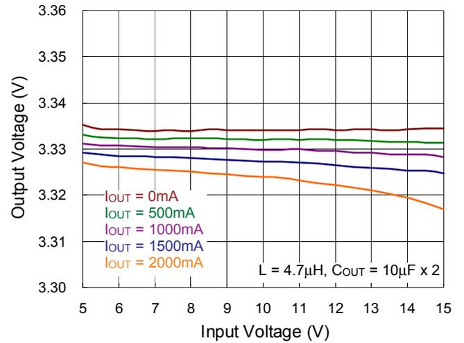
CH2 Buck Output Voltage vs. Input Voltage
