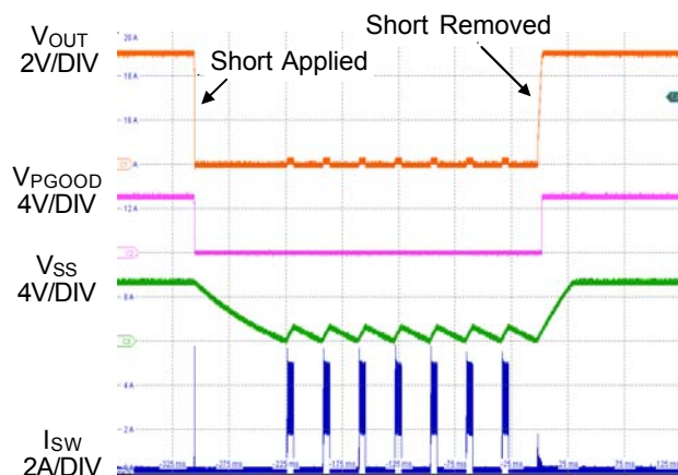
Figure 3. Short-Circuit Protection and Recovery
