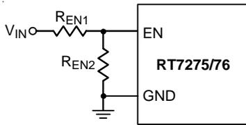
Figure 3. Resistor Divider for Lockout Threshold Setting
