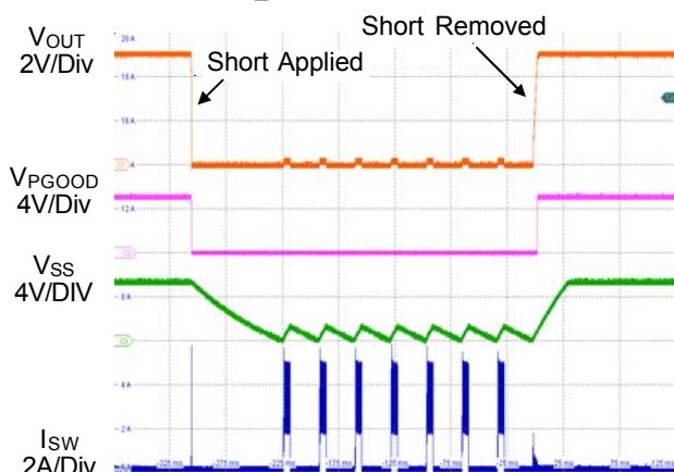
Figure 3. Short Circuit Protection and Recovery
